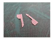
Using a glue stick gently attach the cut out part of this sheet to a piece of 0.12mm brass sheet. Due to the small nature of the parts I find it easiest to score along the red lines with a sharp modelling knife before cutting out the parts using tin snips or strong scissors. Now remove the templates and clean off any remaining glue.
