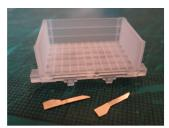
Form the parts by folding the metal through 180 degrees along the fold line. This is best achieved using a hold-and-fold (or similar tool) to fold to just over 90 degrees and then with your fingers to fold the rest of the way. To get the part nice and flat simply squeeze the fold using the hold-and-fold.
